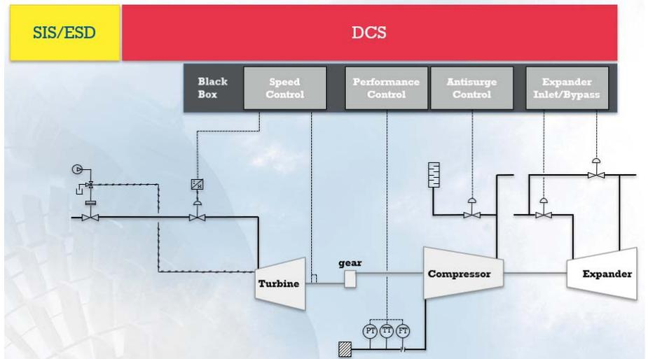
Fig. 1a TMC separate from an Integrated Control & Safety System (ICSS), DCS and/or SIS.
