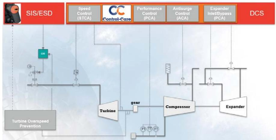
**Fig. 2a** TMC implemented in an Integrated Control & Safety System (ICSS), DCS and/or SIS.
